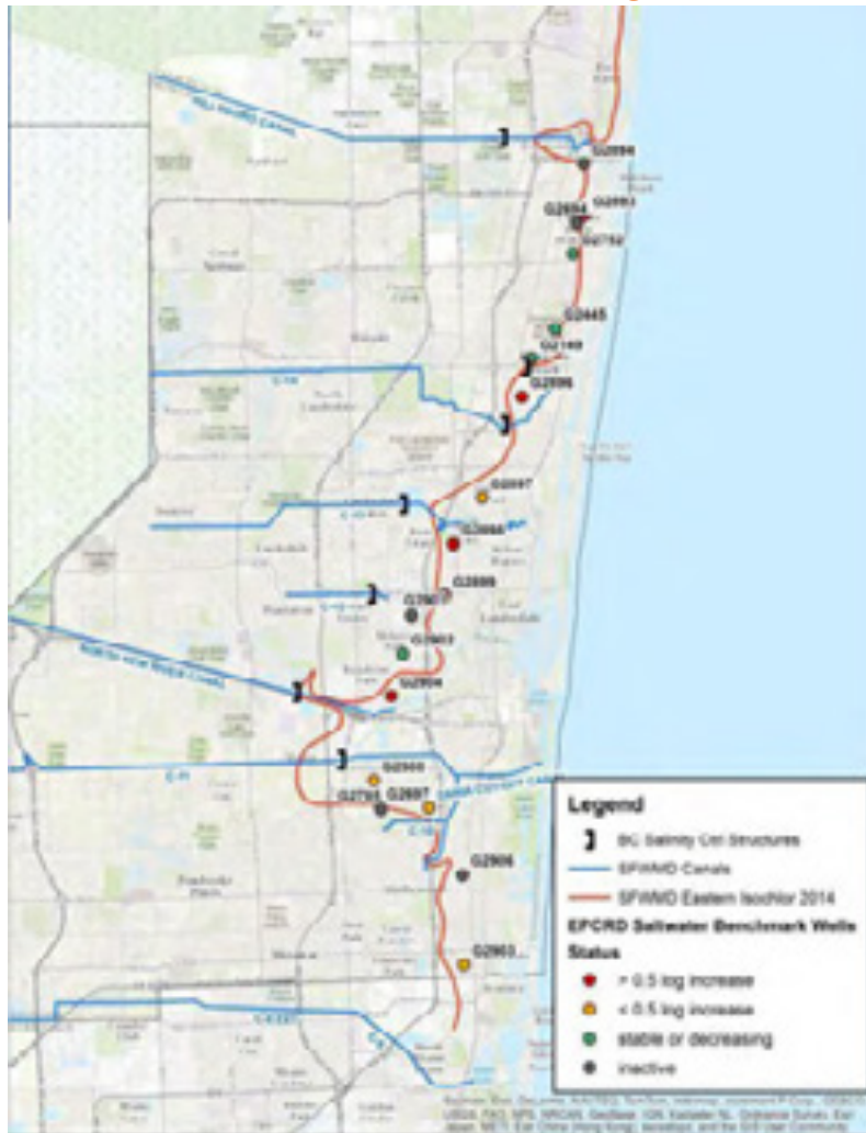
Figure CC-12 Saltwater Intrusion Line and Saltwater Monitoring Wells in Broward County
