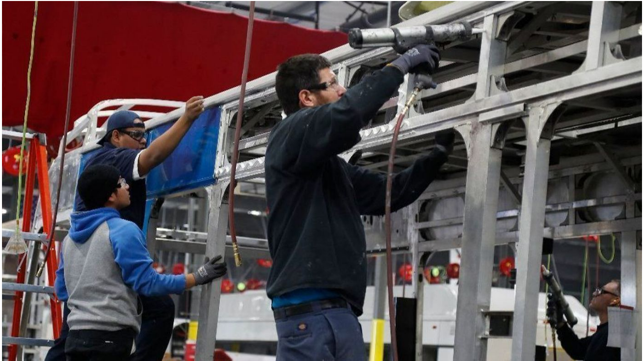
BYD assembly plant worker Jesus Martin applies glue before an aluminum skin is placed on the exterior of an electric bus at the BYD production facility in Lancaster. (Mel Melcon / Los Angeles Times)
