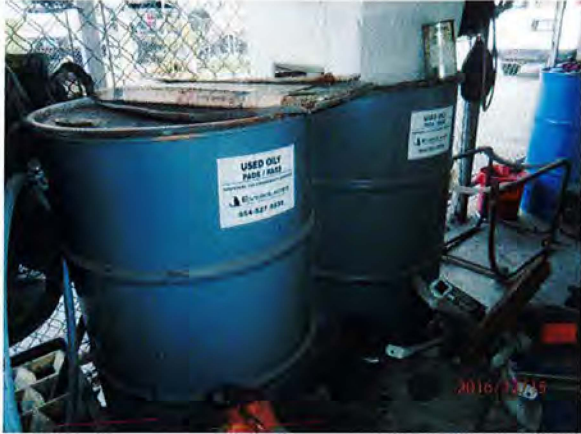
improperly labeled used oil drums
