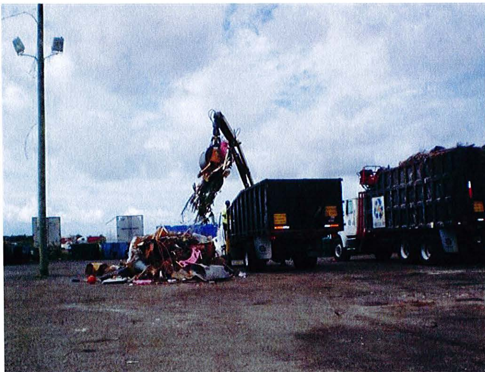
Notes: Grapple truck removing waste pile from the floor
