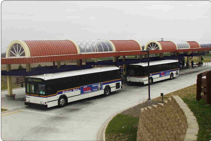
Figure 5.5.3 - Photo - Parallel Bus Berth
