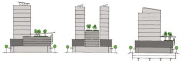
Three diagrams illustrate the integration of parking structures: (from left to right) above grade parking insulated with active uses at the street side and landscape screen on the backside; above grade parking insulated with active uses; and below grade parking using slurry-wall technology with active uses at grade and above.
