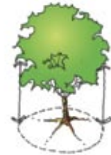
The critical root zone is related to the drip line of the tree.
