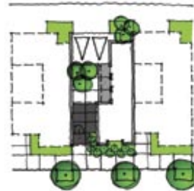
Plan diagram of entry courtyard type infill development with alley access to carport.
